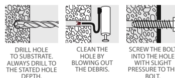
DRILL HOLE TO SUBSTRATE. ALWAYS DRILL TO THE STATED HOLE DEPTH.
